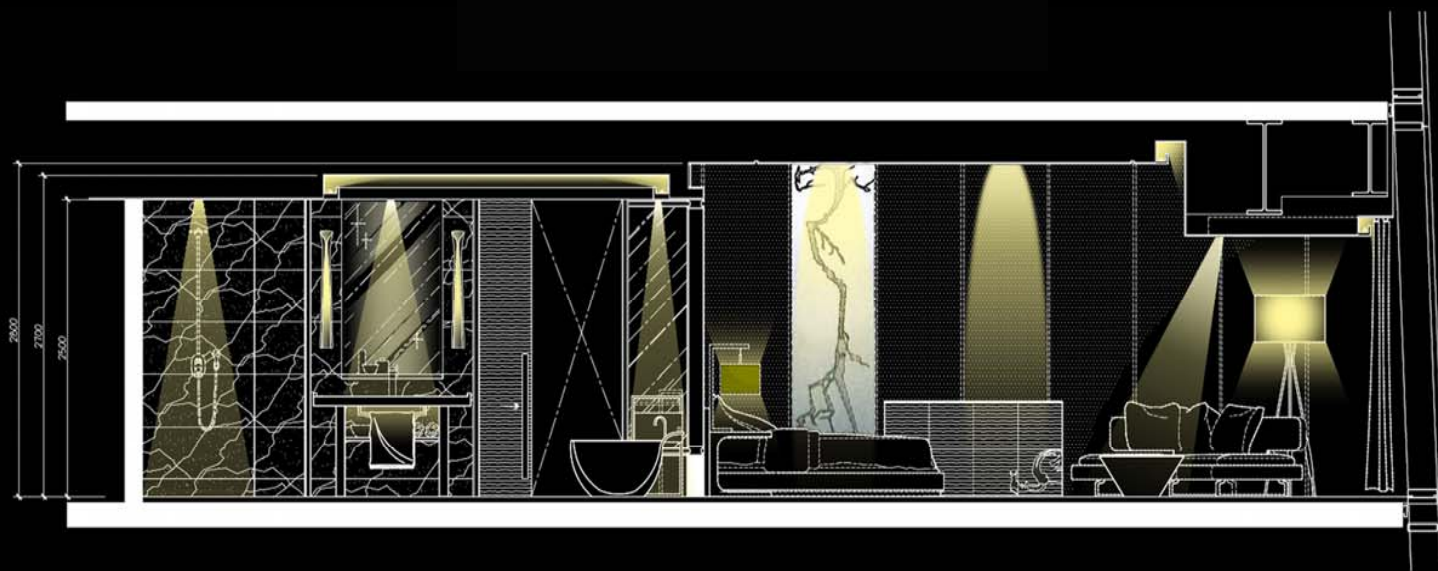
双人客房照明立面图 KING ROOM LIGHTING ELEVATION
